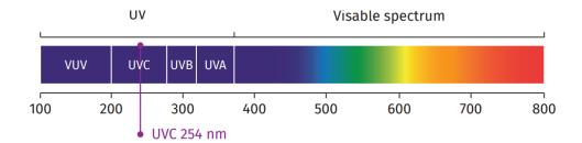
SCU-UV primary function is to neutralize pathogenic organisms and harmful chemical compounds in the supply air. The key principle is based on using ultraviolet germicidal irradiation (UGVI). UGVI is is electromagnetic radiation which inactivates microorganisms and its ability to reproduce by causing photochemical change in nucleic acids.
